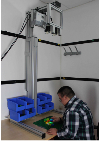
Figure 1: An assistive system supports workers using in-situ projection and detecting micro tasks using a depth camera [1]
